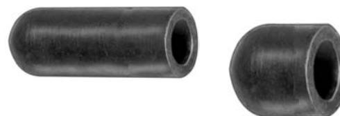
**Screw Grommets:** A variation of the nylon nut. They are used with metal tapping screws throughout the vehicle (interior and exterior). They're installed in a pre-punched hole or slot in sheet metal. The tapping screw cuts its own thread as it's installed. They are mostly found in Japanese cars.
