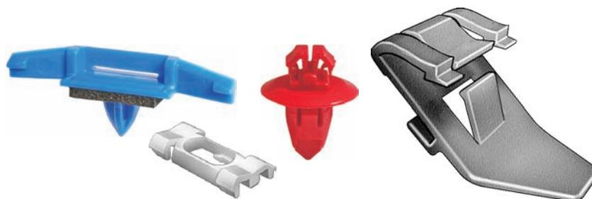
**Nylon Nuts:** Used with metal tapping screws throughout the car (interior & exterior) for attachment. As a tapping screw is installed, it cuts its own thread and spreads the bottom part of the nut apart thus securing it in place. Nylon nuts can be found in door panels, headlight/front-end applications, license plate brackets, arm rests, instrument panels and many other areas.
