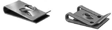
**Universal Moulding Fasteners:** A universal type of fastener for attaching older style mouldings that have lips or curls on the underside. The spring steel arm provides the tension holding the moulding strip. With the perforated plate type, you can break off the plate at 1/16" intervals to fit the moulding. You need to be able to access the back of the panel so you can install a hex nut.
