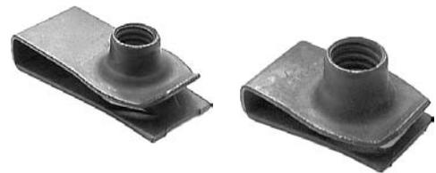
**Flat Nuts:** Made of spring steel and used where the other side of the panel is easy to reach. They can be for either stud type or threaded fasteners. They are used throughout the car under the dashboard, in door panels, trunk area, fenders, etc.
