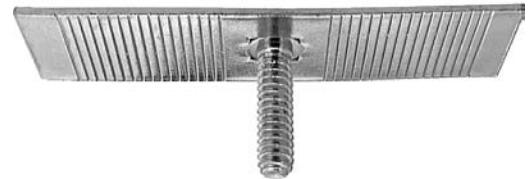
**Washer Head:** A screw/bolt with the washer permanently attached to it. Also called flanged head. The washer head eliminates the need for a separate washer while increasing the load bearing area of the head. Used under the hood, on fenders, doors, front end applications, etc.
